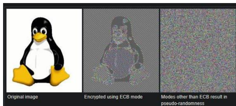
Figure 1: Tux the Penguin Encrypted in ECB vs Pseudo-Random Encryption: Source github picoctf-2019-solutions/Cryptography/aes-abc/readme.md
